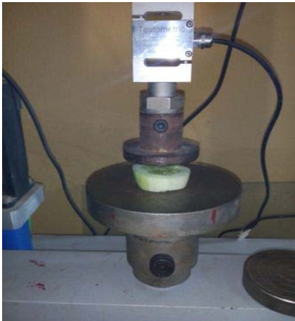
Figure 2: Cucumber fruit undergoing quasi compressive test using Universal Testing Machine (Testometric model, series 500-532)
